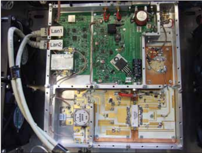
Figure 5 • The internal module of the SNA-based S11-locked microwave power generator.
