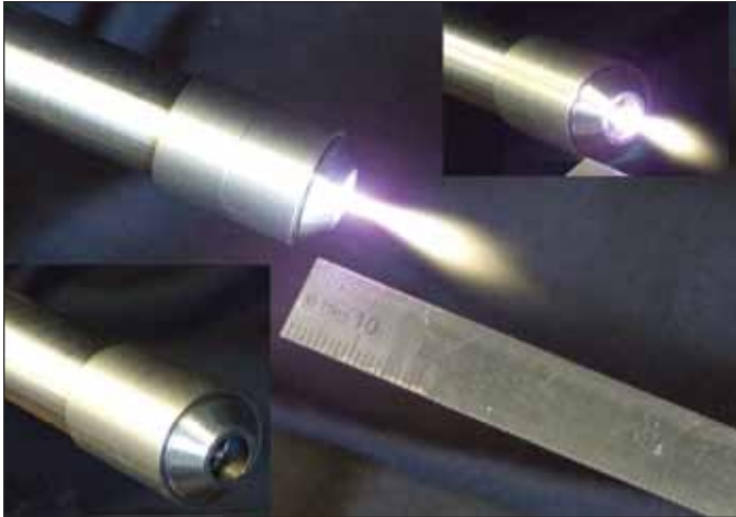
Figure 2 • Microplasma driven by a 200W S11-locked microwave power generator.
