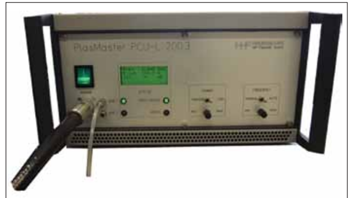
Figure 3 • SNA-based 200 W S11-locked microwave power generator from HHF.
